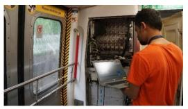
2. MTR and contractor staff have been using the "signalling system simulator" specifically designed for the signalling replacement project for urban lines to simulate various scenarios for testing.
